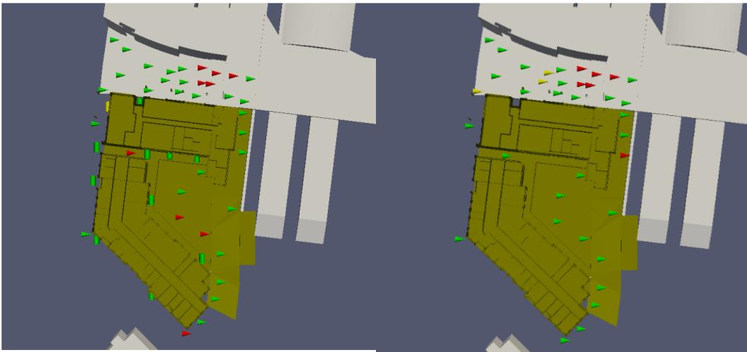
**Figure 5.6: Comparison of Lawson Comfort Criteria on Bridge Street and Dargan Street without (left) and with mitigation (right)**
